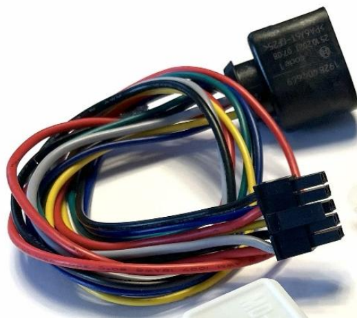
Connection cable to the lambda sensor and power supply
